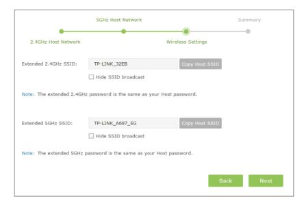
6) Verify your wireless settings and click Finish. The corresponding LED(s)(2.4GHz or 5GHz) should turn on.
